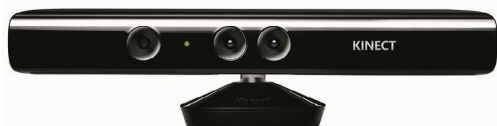
Fig. 1 Microsoft's Kinect has four sensors: a camera, an infrared projector which emits random patterns to recognize the depth of an object, an infrared camera which captures the patterns, and an array microphone to capture voices.
